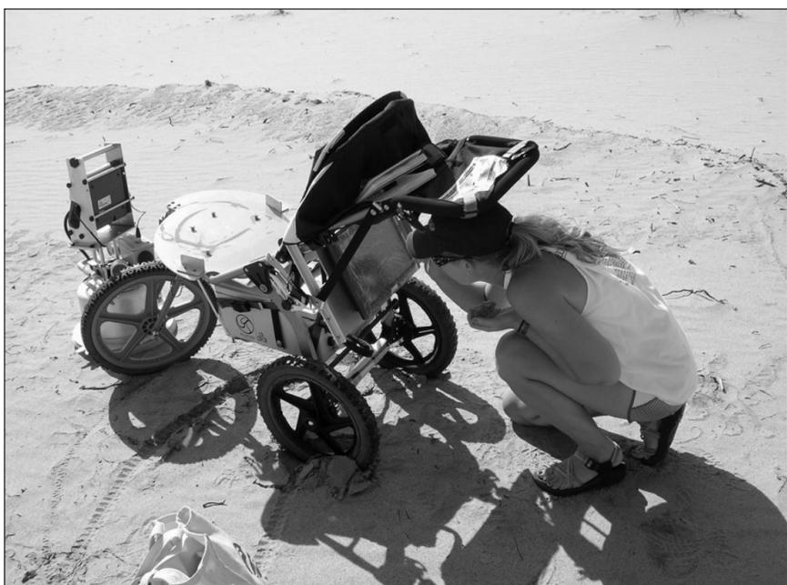
USD undergrad Karen Herrig uses a PI-SWIRL to measure the amount of dust being emitted from an area sandbar.
