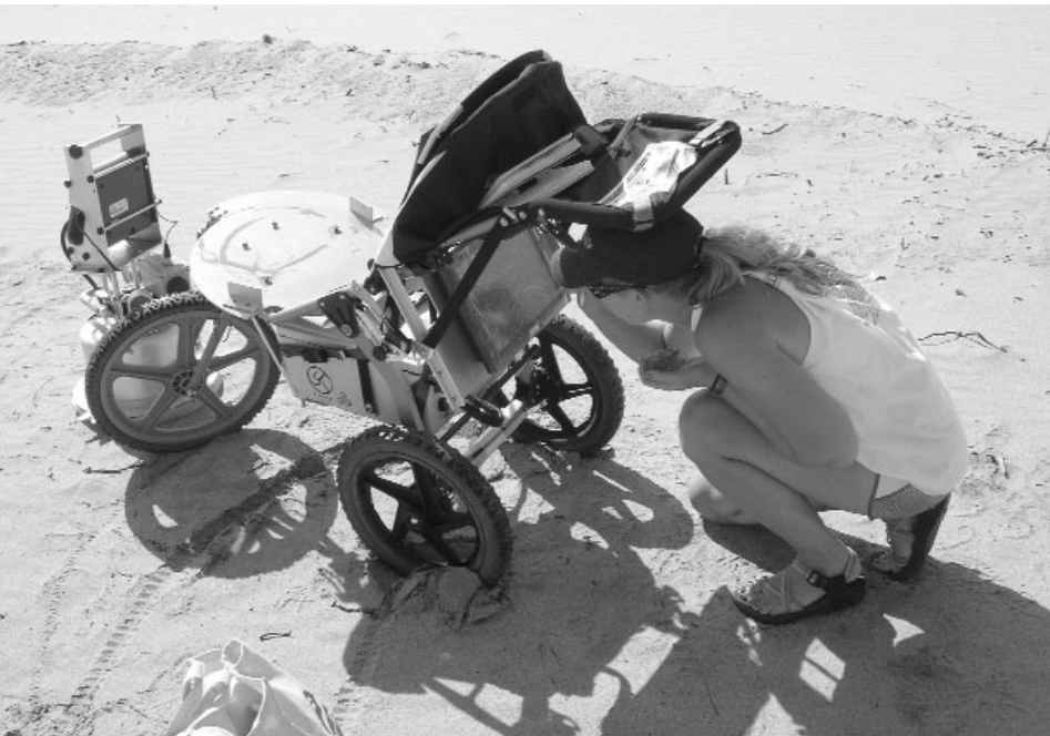
USD undergrad Karen Herrig uses a PI-SWIRL to measure the amount of dust being emitted from an area sandbar. (Courtesy photo)
