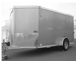
2-3.5K rubber torsion axles, cargo doors or full width ramp, numerous options 6'7" x 12' $6,295 6'7" x 14' $7,995 6'7" x 16' $8,595
