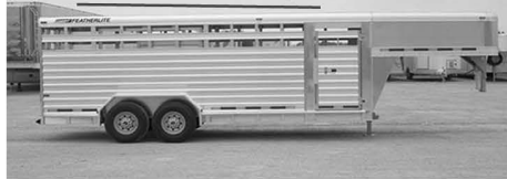
2-7K Torsion Axles, center gates w/slider, rear gate w/inside or outside slider, anti-slip extruded aluminum flooring, 20' $15,495 24' $16,495 30' $20,995
