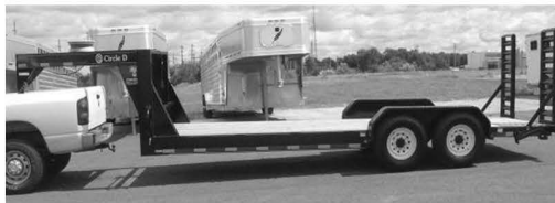
2-6K rubber torsion axles w/EZ lube, 2' beavertail, spring assist rear ramps, rear support legs 20' $5,695 22' $6,295
