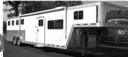
All Aluminum Construction, Rubber Torsion Axles, walk thru door, side escape door, rear fold up tack, awning, 9' Living Quarters pkg. includes: fridge, microwave, large shower, stool, stove, a/c & more 4 Horse $36,995
