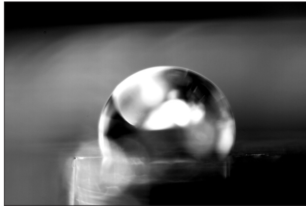
COURTESY PHOTO The above droplet is one photographed and the contact angles measured this summer during Erika Moen and Liz Butler's internship at USD.
