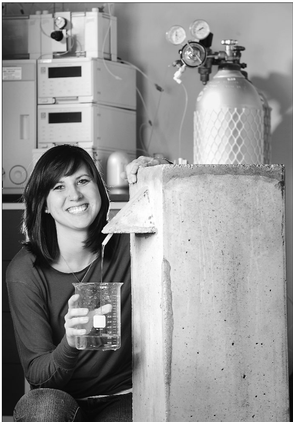
Stacey Joy demonstrates a bio sand filter in an environmental engineering laboratory at the Scott Engineering Center at the University of Nebraska-Lincoln on Thursday, Dec. 15, 2011. Joy was a member of UNL's chapter of Engineers Without Borders, which taught people without access to clean water in Madagascar how to make, install and use the filters.
