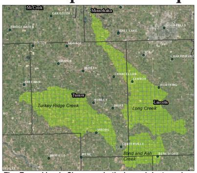
The Turner-Lincoln-Clay organization's goal is to reduce flooding on the lower Vermillion River by increasing soil infiltration and water retention upstream.
